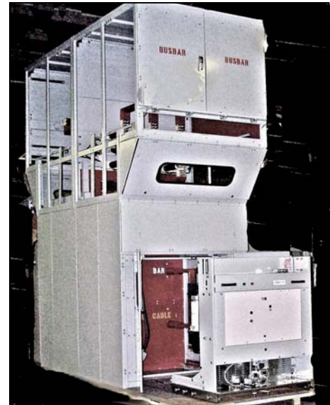
View of switchgear with circuit breaker , after assembly in PACS' factory.
